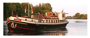
Ex freight barge carrying beer Former purpose: Year of construction: 1921 Dimensions: 81ft (24.6m) x 14ft (4.26m) Generators: 1 x 220 volt Hawker Siddely generator 125 HP DAF (2012) Main Engine: Maximum Speed: 12km per hour Water capacity: 4,940 litres Fuel capacity: 3 tons
